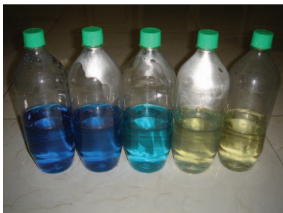
Fig. 9. Photograph of the variation of colors with photocatalytic action.
