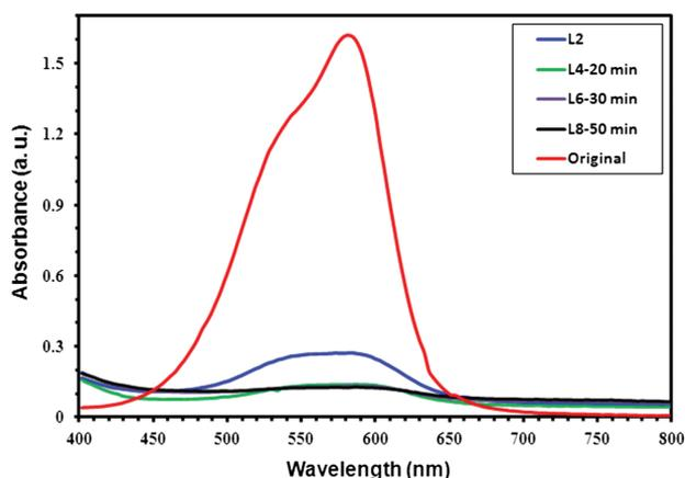
Fig. 3. Visible light absorption spectra of the crystal violet dye solution during photocatalytic degradation due to Indian edible chuna.
