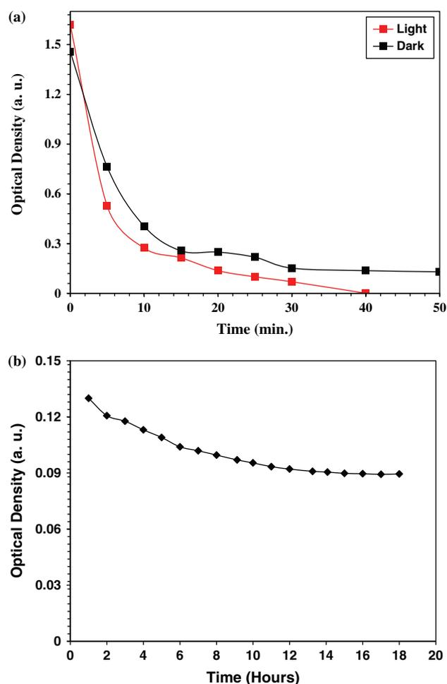
Fig. 4. (a) Variation of optical density at 582 nm for degradation of crystal violet dye in dark and light with Indian edible chuna as photocatalyst. (b) Variation of optical density at 582 nm for crystal violet dye degradation in dark (chemical degradation process) using Indian edible chuna.
