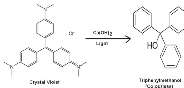
Fig. 5. Possible mechanism for chemical/photocatalytic degradation of crystal violet dye due to Indian edible chuna.
