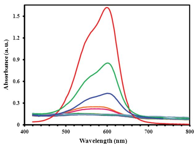
Fig. 2. Visible light absorption spectra of the crystal violet dye solution during chemical degradation by Indian edible chuna in dark.
